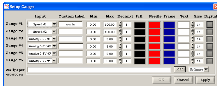
Figure 17: Configure Gauge Inputs (2)
